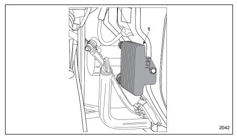
Figure 4-11 Engine Oil Cooler
